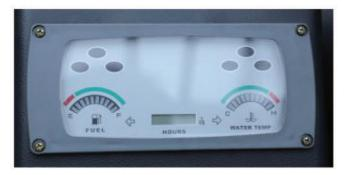
Intelligent instrument panel(fuel level, hour meter, water temperature, engine oil indicator, charger indicator, preheating indicator, oil filter alarm, forward, reverse and neutral direction indicators)
