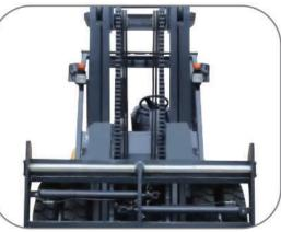
Heavy duty welded mast: Wide designed with good visibility, ensures its excellent forward visibility, improves working efficiency and safety.
