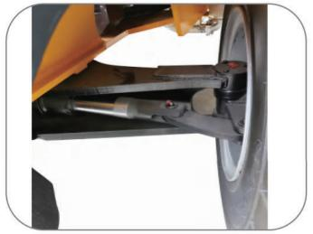
Strengthened and tough axles & large turning angle: Make it efficient and flexible handling and steering.
