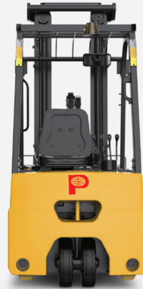
CPD15TVL Length to face of forks: 1813mm(L2) overall width: 1070mm(b1/b2)
