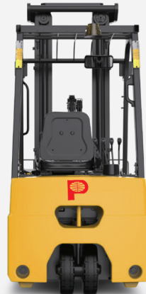
CPD18TVL Length to face of forks: 1913mm(L2) overall width: 1070mm(b1/b2)
