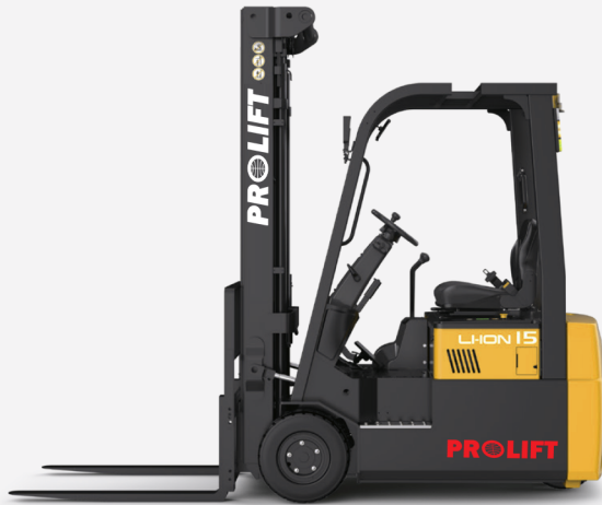
CPD15TVL Length to face of forks: 1813mm(L2) overall width: 1070mm(b1/b2)
