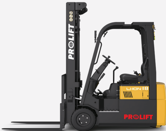
CPD18TVL Length to face of forks: 1913mm(L2) overall width: 1070mm(b1/b2)
